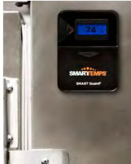
**SMART TEMPS** The Mishawaka company's technology monitors the temperature of things that need to be cold or hot, and automatically sends out email, text or phone alerts if a sensor senses that something isn't the way it should be.
