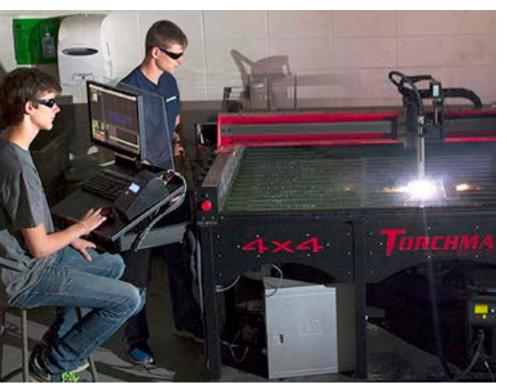
**BEST UNIVERSITY FOR OBTAINING A TECHNOLOGY DEGREE Purdue University** Northwest. Pictured here are technology students at the Calumet Campus in Hammond using an advanced-manufacturing plasma torch to produce parts for an off-road vehicle.
