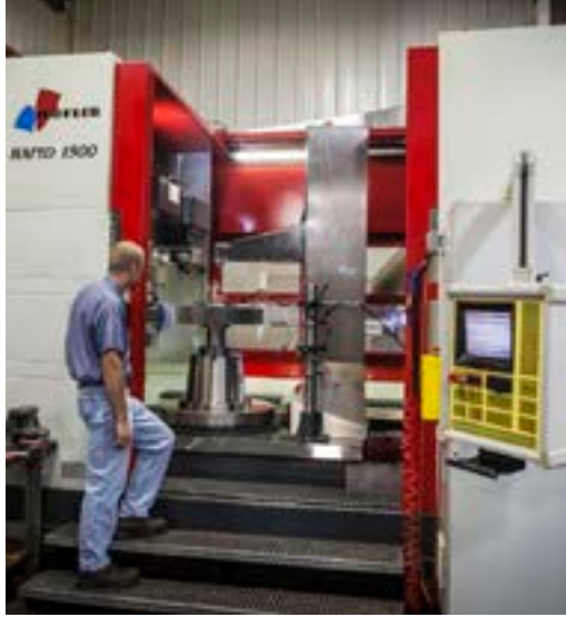
"CONSTANTLY REINVESTING" Schafer Industries, based in South Bend, makes gears and axle assemblies. Pictured here is a gear grinder.
