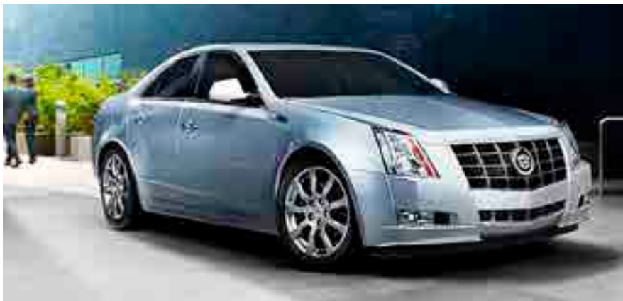
FAST CAR With a 556-horsepower V8 engine, the Cadillac CTS can hit 60 mph in under 4 seconds, and oversized Brembo brakes help it stop quickly, too.
