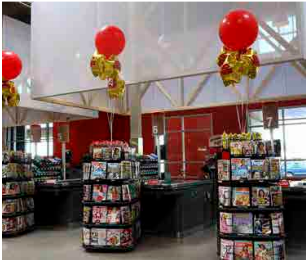
CHECK IT OUT Skylights and windows let in natural light at the Strack & Van Til store in Cedar Lake, cutting lighting usage in half.
