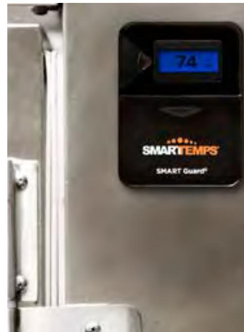
**SMART TEMPS** The Mishawaka company's technology monitors the temperature of things that need to be cold or hot, and automatically sends out email, text or phone alerts if a sensor senses that something isn't the way it should be.
